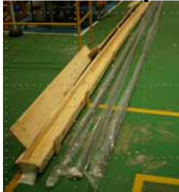
10 meter-long double-wall tube with wire mesh
