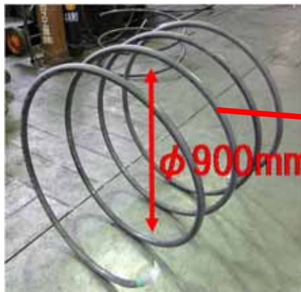
Helical-coil processed tube of welded double-wall tube
