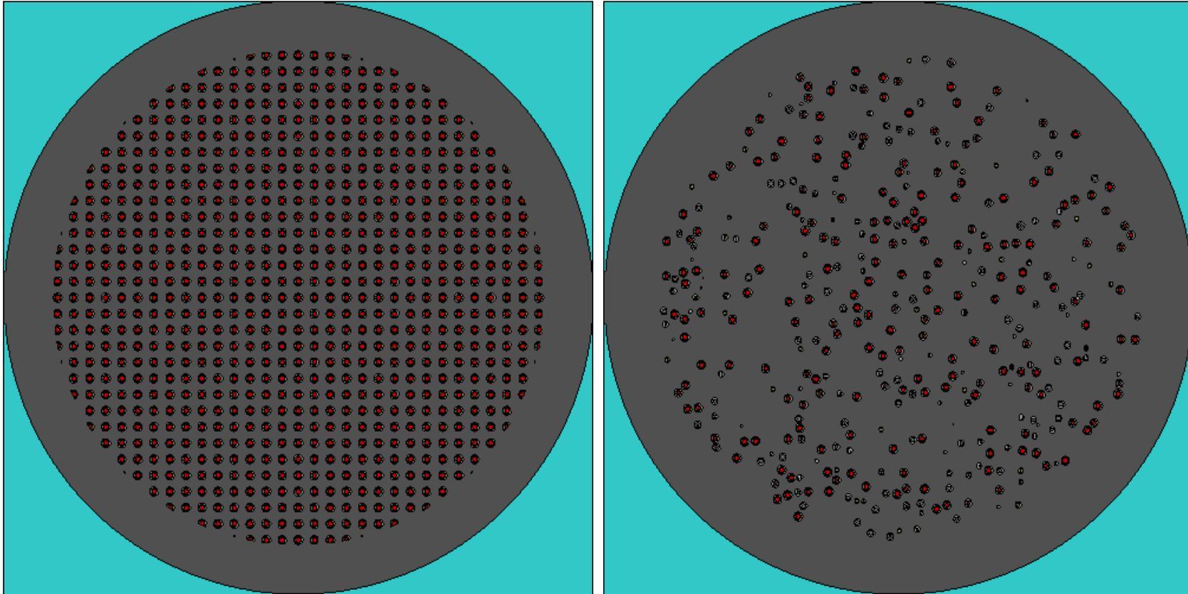
Left: PBMR fuel pebble with regular lattice model for particle distribution.
