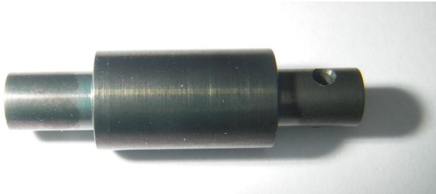
Visual appearance of CrN coated sample after exposure to supercritical water
